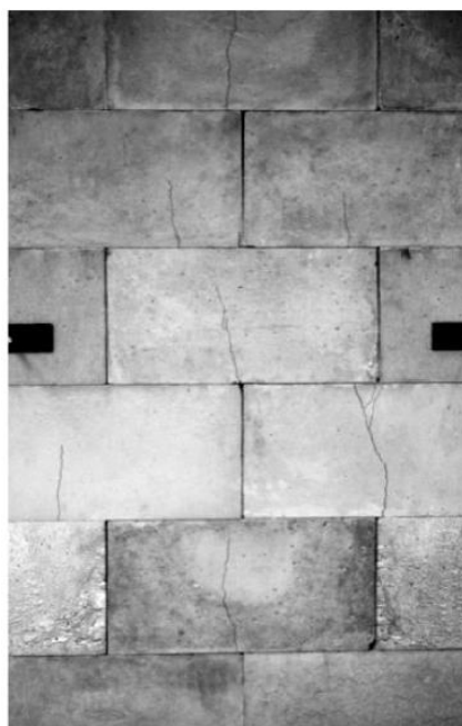
Figure 18 Characteristic crack patterns observed during experimental investigations involving vertical loadings and bending moments on stretcher-bonded and dry-stacked masonry structures
