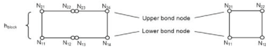
Figure 3 Definition of nodes of full and half masonry elements
