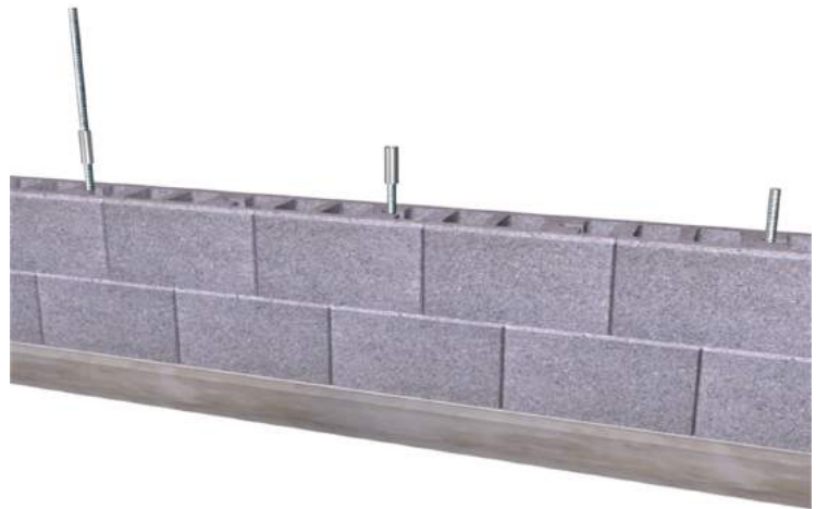
Fig. 4.19 Placing the Stop-Type Couplings
