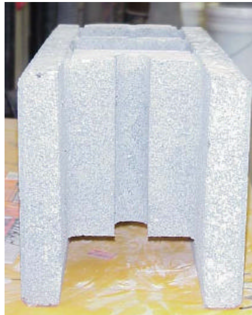
Figure 2—Flexlock CMU Showing Compression Testing Orientation
