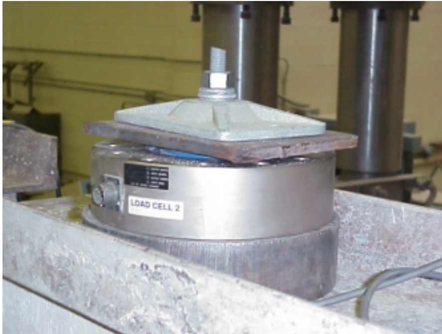
Figure 6—Load cell setup for tensile load measurement
