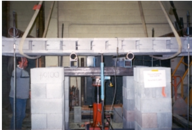
Figure 7—Test Setup for Third-Point Loading
