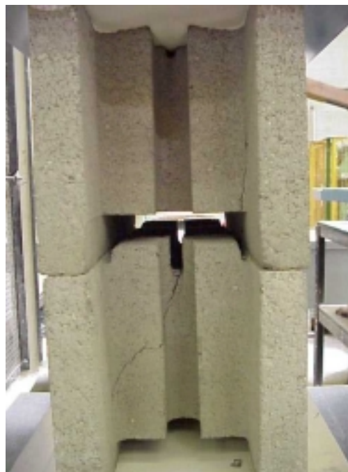
Figure 4—Web crack at 30,000 lbs, test no. 2
